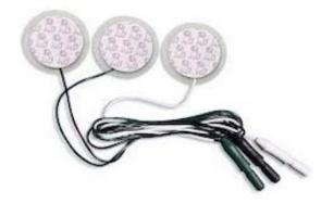
It stick to chest for picking up ECG signals. The centre is filled with liquid electrode gel for good contact and pickup. Remove plastic backing sheet to expose the adhesive. Then affix to chest and connect wires to your ECG module for signal pickup. Gives good stabilization and quick reading.
